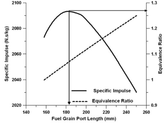
**Fig. 6 Variation of vacuum specific impulse and equivalence ratio with fuel grain port length.**
