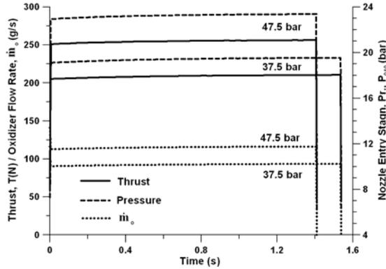
**Fig. 2. Performance prediction for different pressures in H<sub>2</sub>O<sub>2</sub> propellant tank.**
